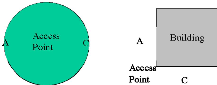
Figure 4. Increased collisions due to the hidden node problem reduces overall wireless LAN performance, and cannot be prevented by channel planning.
