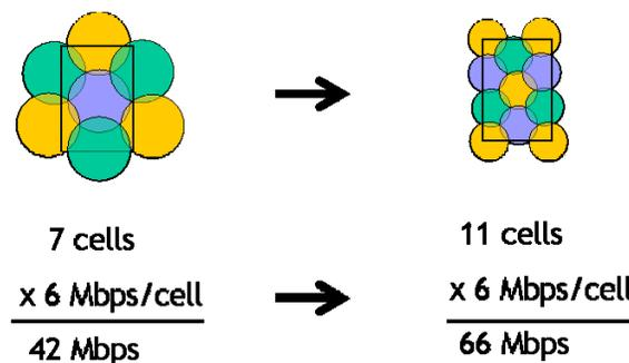
Figure 2: A microcell deployment increases the number of access points in a given area by reducing transmit power. It is widely recommended as a method to create more bandwidth for higher densities of clients.
